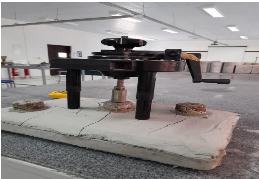
Figura 13: Pull off test
