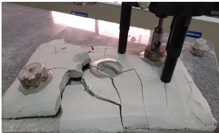
Figura 14: Pull off test
