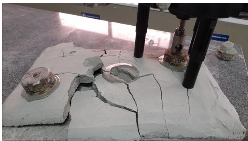
Figura 27: Pull off test
