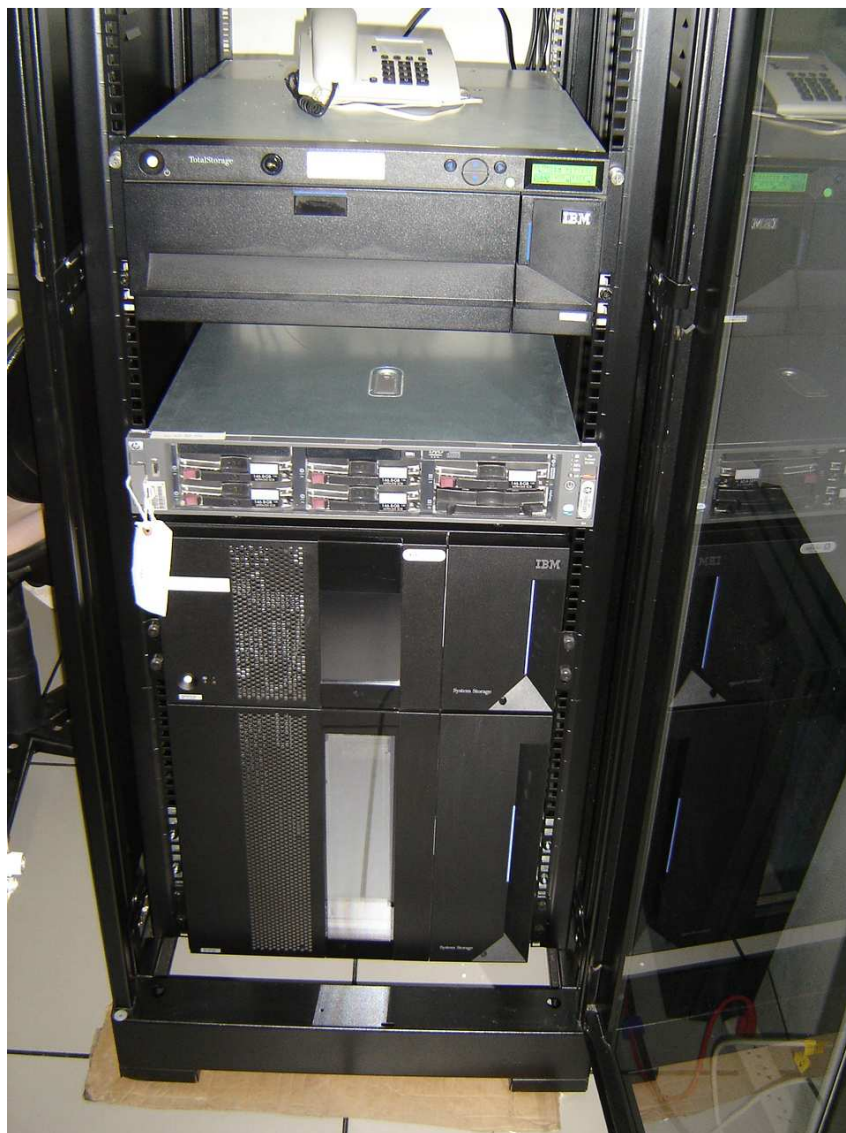
Figura 35: Rack com Tape library IBM ULT3582, Servidor TSM e Tape library TS3310.
