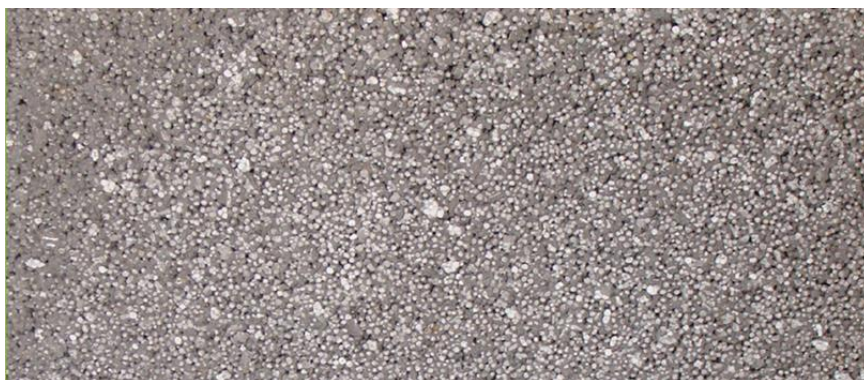
Figura 10-Concreto leve com EPS.
