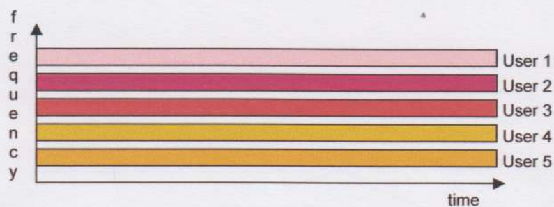
Figura 2: FDMA - frequency division multiple access . Fonte: PIRTTIAHO, 2001
